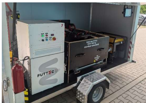
Machine assembly with microwave furnace FF-9 (third generation)
